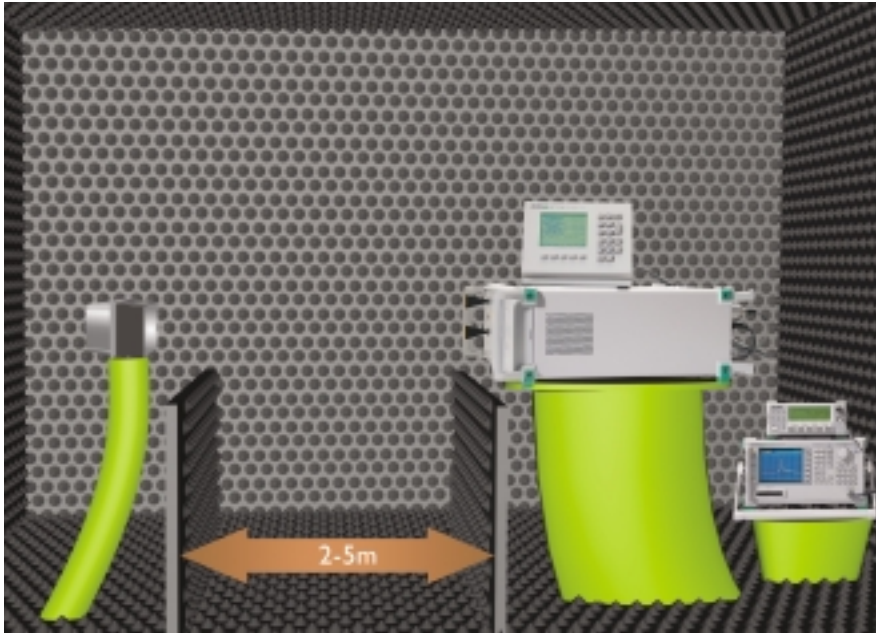
Anechoic Chamber Measurement Setup
